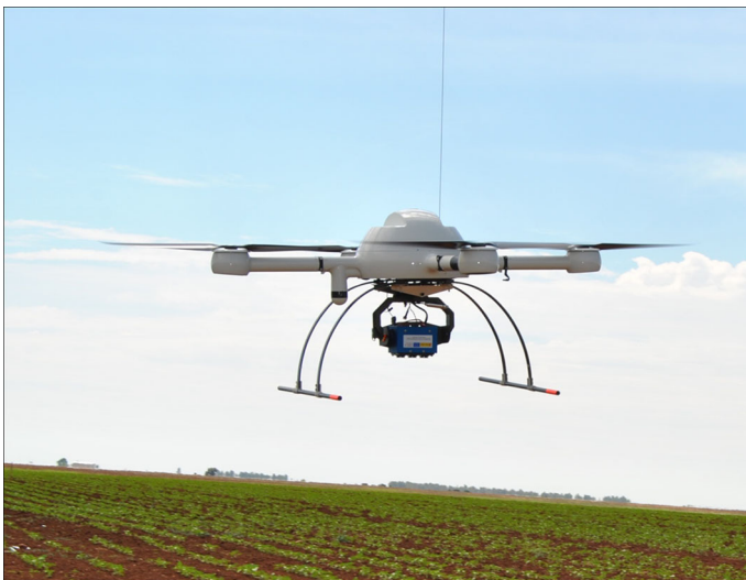
Fig. 1 Microdrone MD4-1000 with the multi-spectral camera (6 channels) embedded flying over one the sunflower experimental fields
