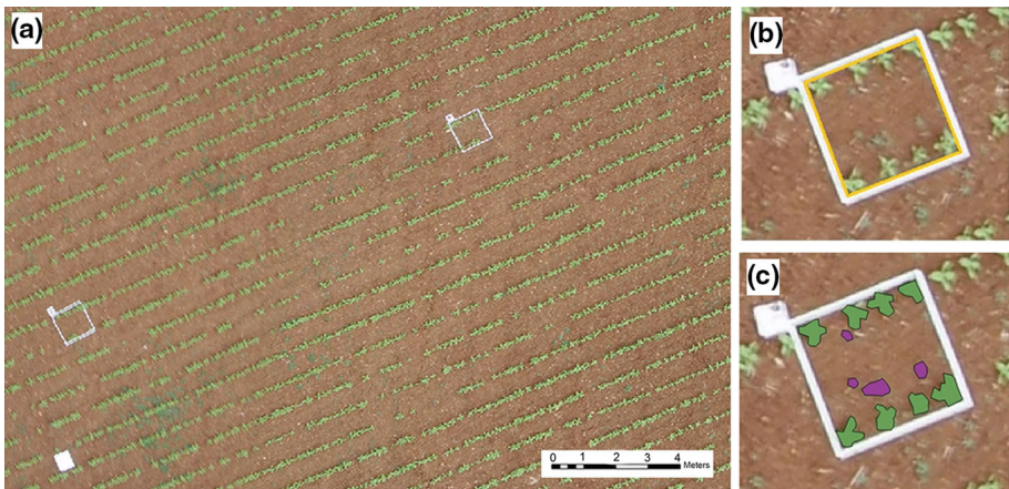
Fig. 3 a Partial view of the ortho-mosaicked imagery at 30 m altitude (sunflower field 2), showing the sunflower rows, the spectralon ( white square placed between two sunflower rows at the bottom-left ), some patches of weed infestation and some of the 49 1 × 1 m square frames ; b Detail of vector file created for every square frame ( yellow ); c detail of the vector file created for the sunflower crop ( green ) and weed ( violet ) classes in one the 49 square frames
