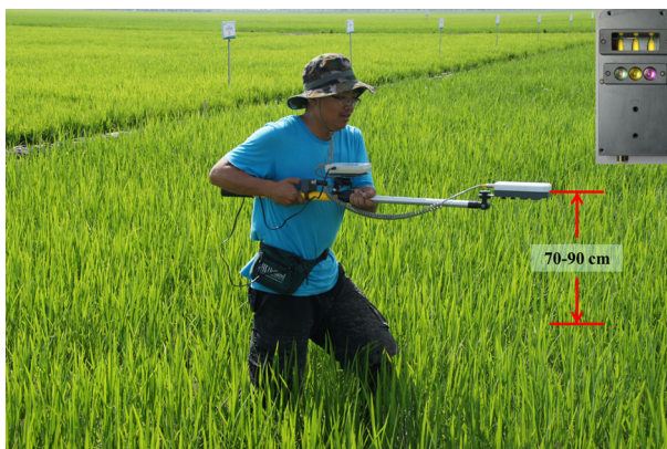
Fig. 1 Collecting rice canopy reflectance data using Crop Circle ACS-470 active canopy sensor
