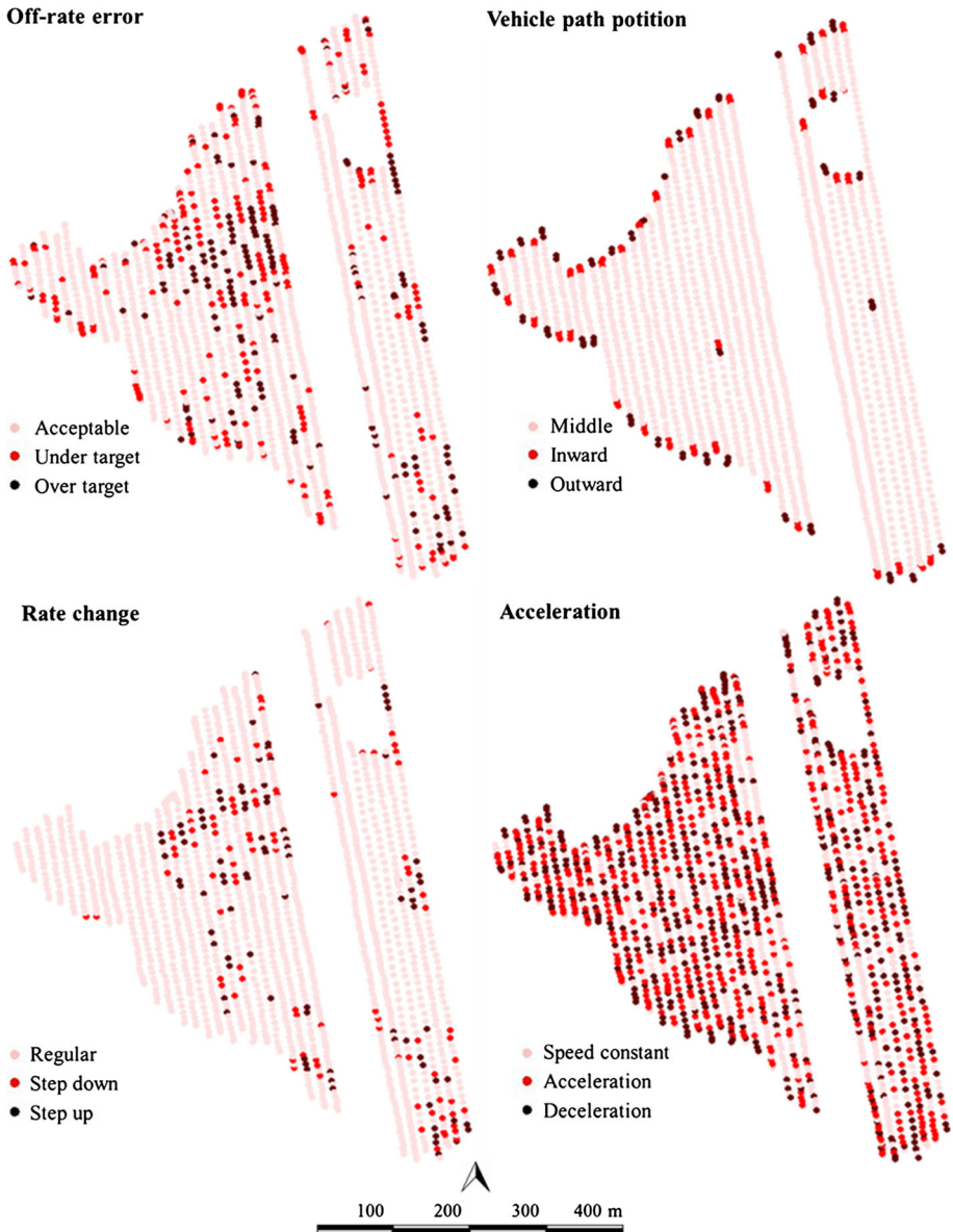
Fig. 5 Maps of off-rate error and possible error source classification on a corn field fertilization
