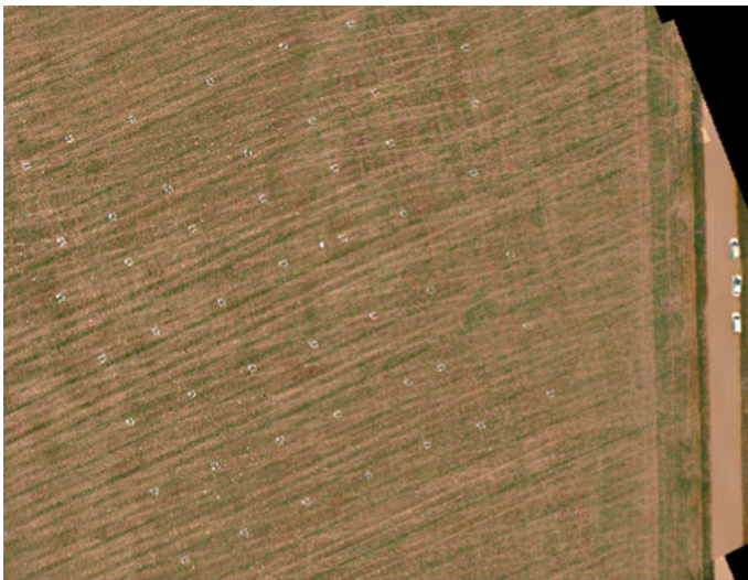
Fig. 4 Example of the resulting orthomosaics of the 100 m altitude flight at Monclova; 48 white 1 m 2 frames are visible
