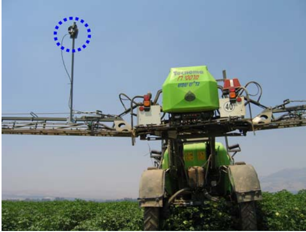
Fig. 2 Infrared scanner mounted on a high pass sprayer
