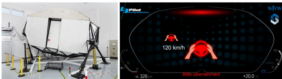
Fig. 1 High fidelity driving simulator (left) and visual request to intervene on the tachometer display (right)
