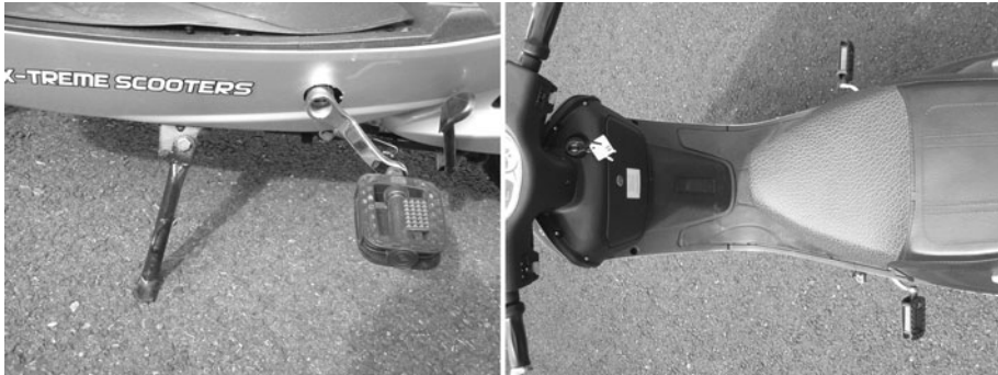
Fig. 6 Pedals on street legal scooter style E-bike in the USA
