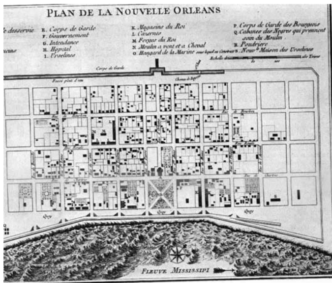
Fig. 1 An example of gridiron layout in town planning of the fortified port city of New Orleans, Louisiana in 1764 (12 years before Captain Francis Light established George Town as a trading centre)
