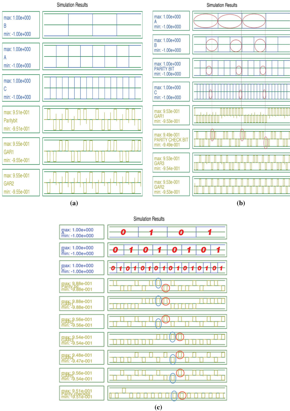
Fig. 13 Simulation results of QCA layout of the a odd parity generator, b odd parity checker, c nano-communication circuit
