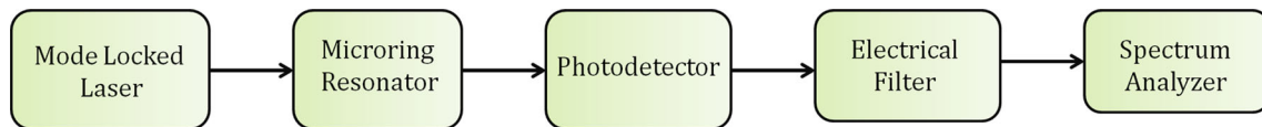
Fig. 2 Block schematic of photonic system for THz generation based on microring resonator and electrical filter
