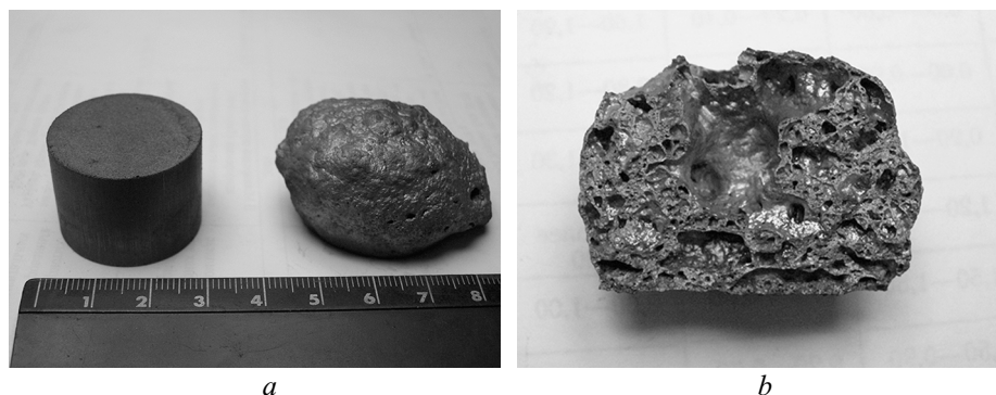
Fig. 1. Appearance of the samples (a) before (left) and after (right) reactive thermal synthesis and macrostructure of the composite (b)
