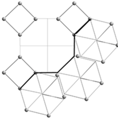
Fig. 2. Interface of \text{LaB}_6 and \text{MeB}_2 atomic planes filled with boron atoms
