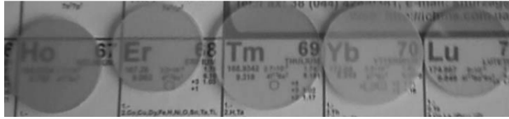
Fig. 4. Transparent ceramics based on C-type pure lanthanide oxides
