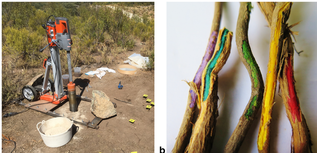
Fig. 2 Photographies from unpublished (Cabal et al.) ecological fieldwork showing the use of a- a construction diamond drilling machine for extracting soil cores by rotation, and b- woody roots
