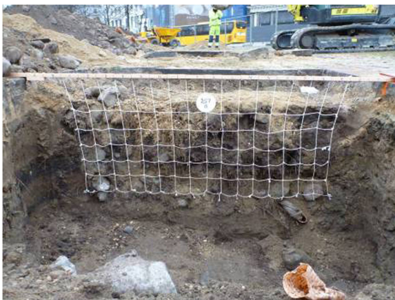
Fig. 3 Measurement setup with grid for root measurements in soil profile. Dimension of squares = 10 × 10 cm
