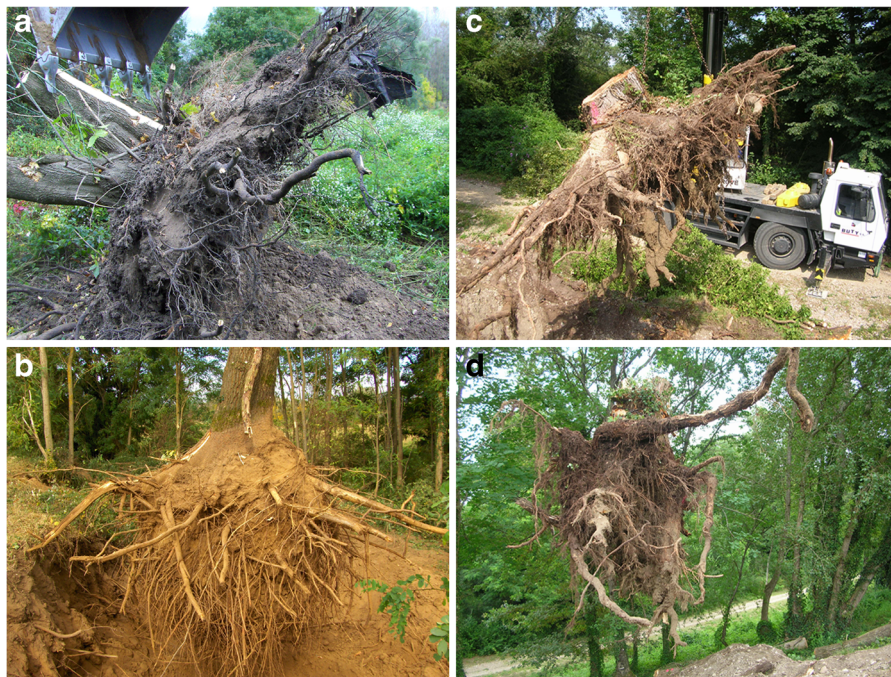
Fig. 2 The four types of root systems. a Shallow root system – Maple at dike toe – Loire River, fine material. b Heart root system – Oak at dike slope middle – Loire, fine material. c Mixed root
