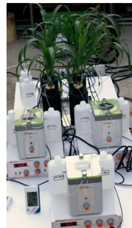
Fig. 2 pH-stat system experimental setup used to maintain constant pH of the exudate collection solutions
