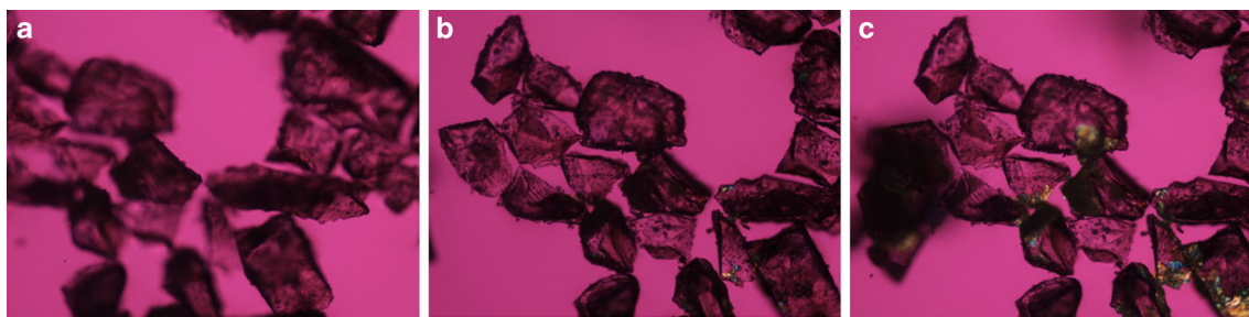
Fig. 11 Polarized light microscope images of neat amorphous CEX exposed to SPB with 5 \mu\text{g/mL} pre-dissolved HPMCAS. (a) unexposed, (b) 5 mins, and (c) 60 mins.
