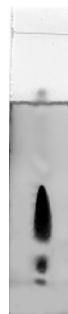
Fig. 5. Chromatogram of sea buckthorn oil EtOH extract (5 \mu L) with gradient chromatography.
