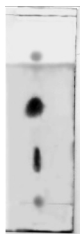
Fig. 4. Chromatogram of Aekol preparation in EtOH (3 \mu L) with gradient chromatography [system 1, hexane:CHCl 3 (19:1), 8-cm run; system 2, hexane:CHCl 3 (3:1), 6-cm run].
