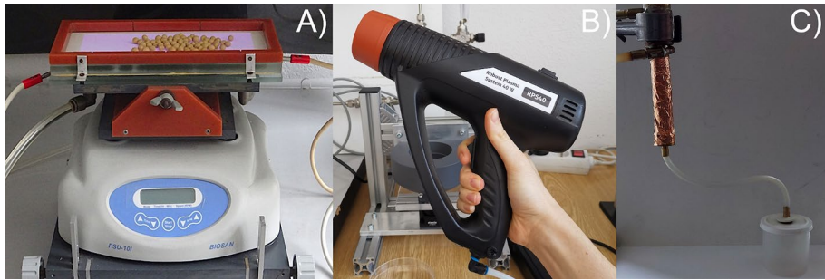
Fig. 2 Photograph of the: A DCSBD plasma source, B MSDBD plasma source, C APJ plasma source
