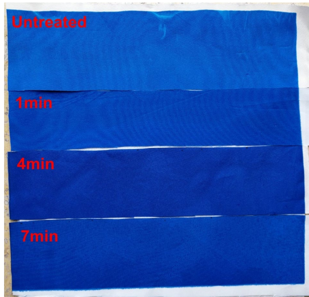
Fig. 10 Photograph of a PET-TiO 2 -S L fabric sample with one-time multiple color printing through different plasma etching time, respectively
