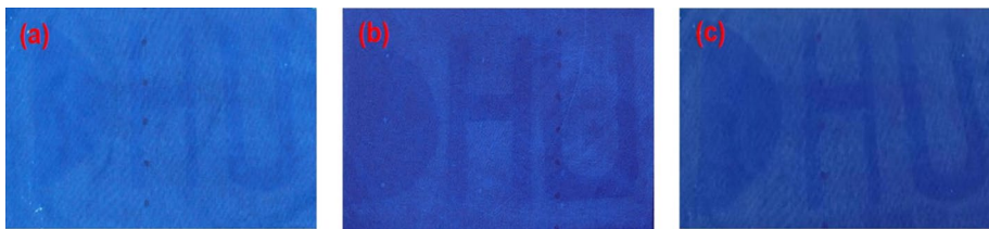
Fig. 11 Photographs of printed fabric samples at 7 min of (a) PET, (b) PET-TiO 2 -S L , and (c) PET-TiO 2 -S H samples, respectively
