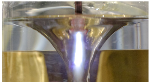
Fig. 4 Typical arc-water vortex interaction; exposure time 1/40 s, aperture f /5
