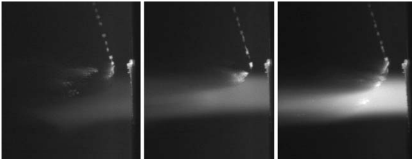
Fig. 5 Influence of the arc fluctuations on drops penetration in the Ar–H 2 plasma jet
