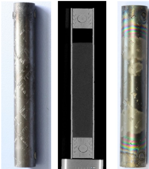
Fig. 14 SiC CMC samples as received (left), X-ray tomography showing end plugs and graphite core (mid), and after 1 h steam oxidation at 1700 °C (right)
