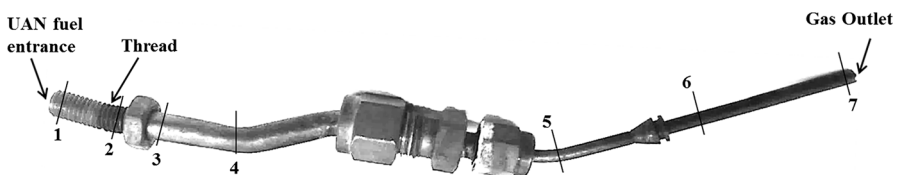
Fig. 2 Side view of the 170-mm-long 316 SS inlet tube in which the aqueous UAN fuel ignition and combustion occurred
