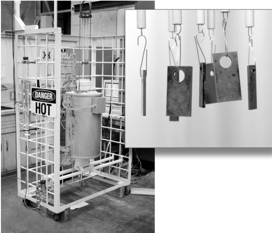
Fig. 3 Cyclic-oxidation apparatus for testing in atmospheric pressure steam/air mixtures
