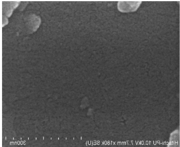
Fig. 6 FESEM image of 60\text{TeO}_2\text{-}15\text{Bi}_2\text{O}_3\text{-}15\text{B}_2\text{O}_3\text{-}10\text{KCl} a glass sample
