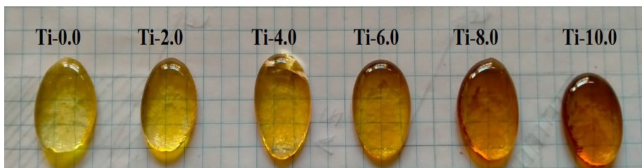
Fig. 1 Photo of the prepared Ti-X glasses
