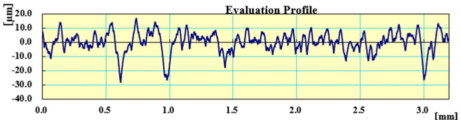
Fig. 17 Surface roughness profile at laser power of 15 W, pulse frequency of 70 kHz, duty cycle of 70%, and scan speed of 5 mm/s
