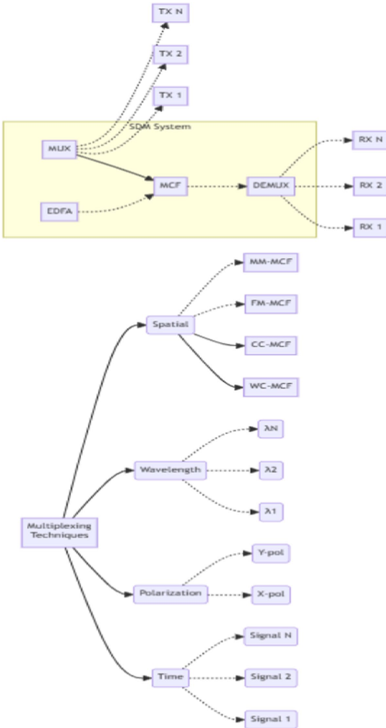
Fig. 3 Schematic diagram of space-division multiplexing (SDM) system and multiplexing techniques
