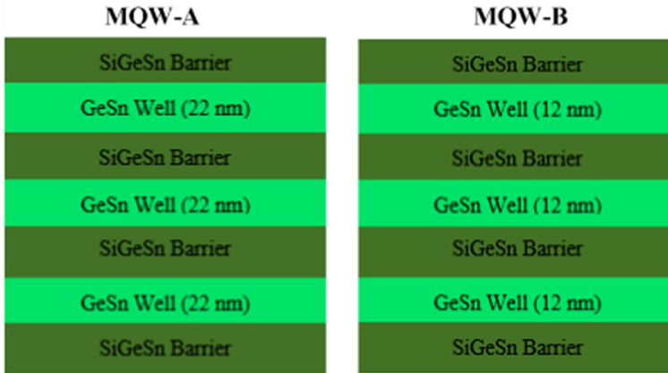
Fig. 2 MQW-A and MQW-B Structure of well width 22 and 12 nm
