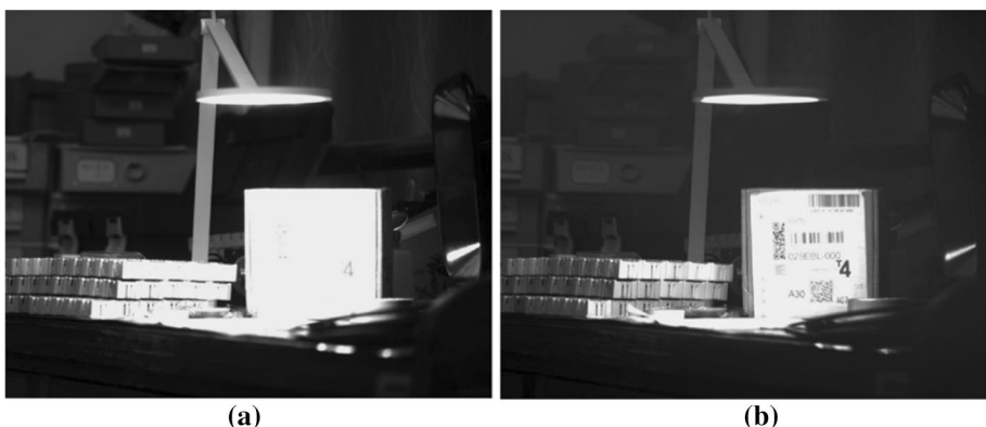
Fig. 7 a Image captured by ordinary camera, b Image captured by ICMOS camera
