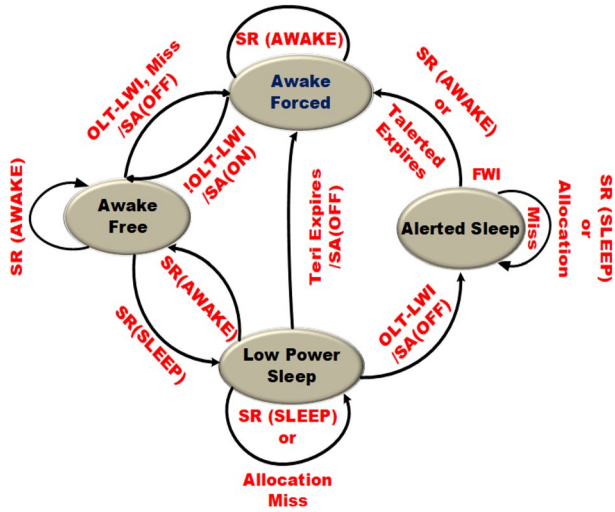
Fig. 5 Cyclic sleep state diagram for OLT
