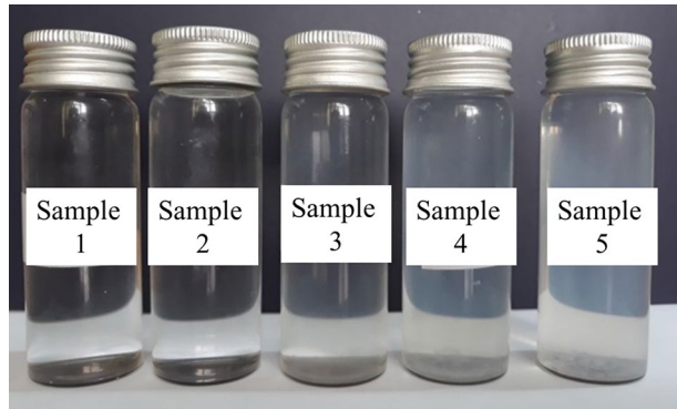
Fig. 1 Cd(OH) 2 /CdO nanostructures suspensions produced by laser ablation
