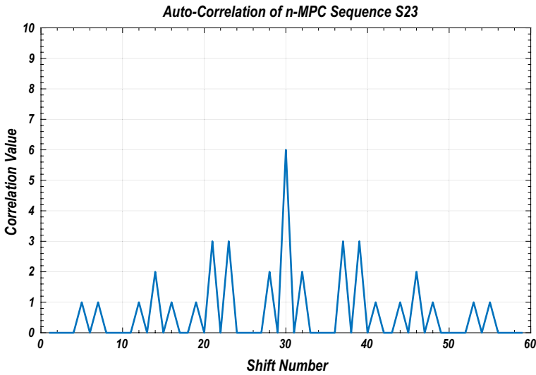
Fig. 4 n-MPC sequence S_{2,3} auto-correlation values when P=5
