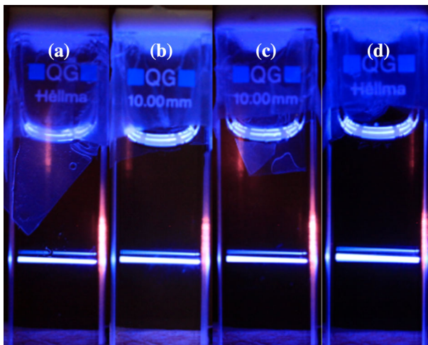
Fig. 7 Photographs of UC luminescence of a 5% \text{Li}^+ concentrations sample, b 10% \text{Li}^+ concentrations sample, c 15% \text{Li}^+ concentrations sample, d 20% \text{Li}^+ concentrations sample for \text{NaYF}_4:\text{Yb}^{3+}, \text{Tm}^{3+} microcrystals under 980 nm excitation at a power > 500 \mu\text{W}
