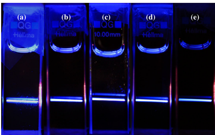
Fig. 6 Photographs of UC luminescence of a pH4 sample, b pH6 sample, c non-modified sample, d pH8 sample and e pH10 sample for NaYF 4 :Yb 3+ , Tm 3+ microcrystals under 980 nm excitation at a power > 500 \mu W
