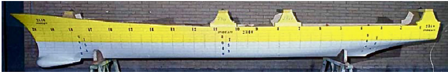
Fig. 1 A 5.720 m length model of the DTMB 5415 (CNR-INSEAN model 2340)
