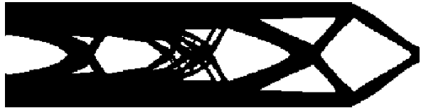
Fig. 19 A beam with dimension 4 \times 1 is discretised using 1564 cells, and a material grid of 800 \times 200 , p = 10 , and the objective stress is \sigma^{obj} = 45
