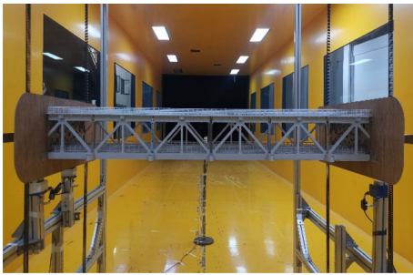
Fig. 5 Section model in wind tunnel
