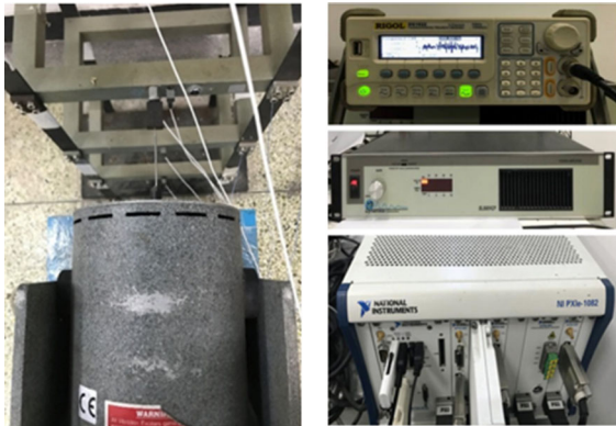
Fig. 12 Electromagnetic vibrator and signal collector
