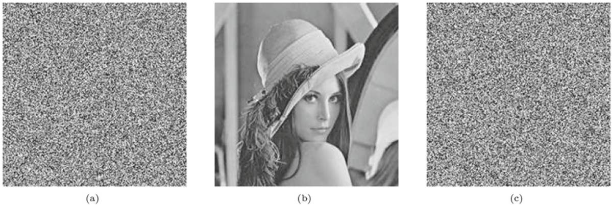
Fig. 10 Results of key sensitivity analysis. a Ciphertext; b decrypted outcome by the initial key; c decrypted outcome by the changed key
