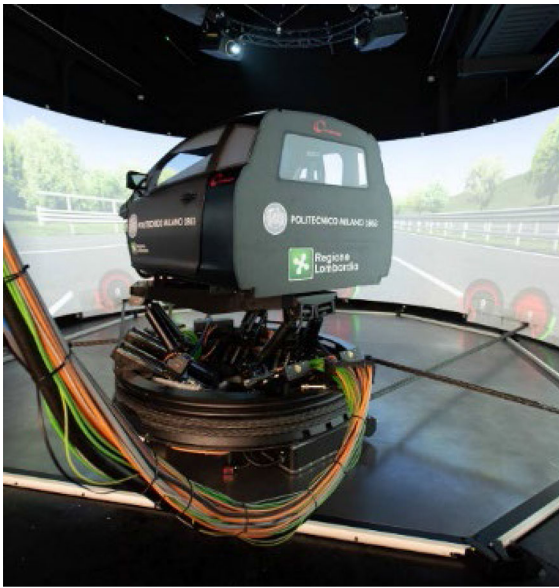
Fig. 5 The driving simulator and the complex car model that were used to validate the results coming from bifurcation analysis of the model in Fig. 1 Data are reported in Appendix A
