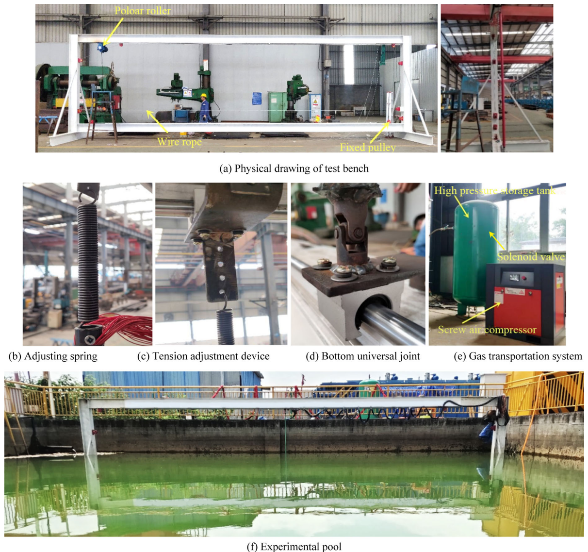
Fig. 4 Physical diagram of test system
