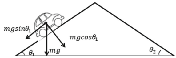
Fig. 1 Schematic of the gravitational force upon a vehicle on the slope gradient
