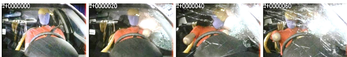
Fig. 1 Occupant struck by the side structure of the car body deforming when hit by the front of another car during a crash test; frames taken every 0.02 s from the beginning of the collision contact [12]
