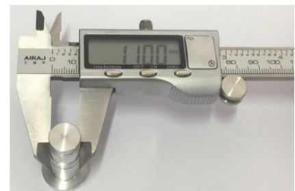
(b) Shaft with clearance value of 0.5mm
