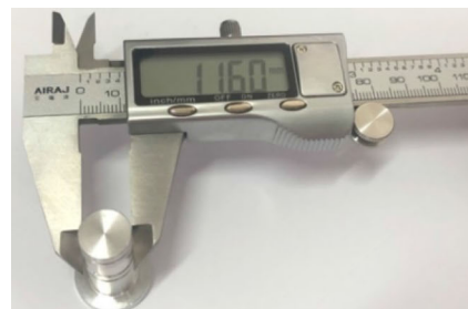
(a) Shaft with clearance value of 0.2mm
