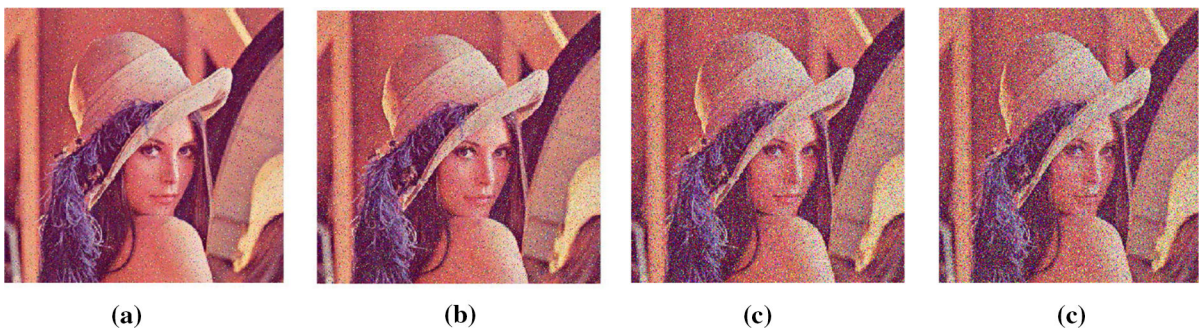
Fig. 27 Decrypted images attacked by salt and pepper noise with different noise densities. a noise density is 0.04, b noise density is 0.08, c noise density is 0.16, d noise density is 0.2
