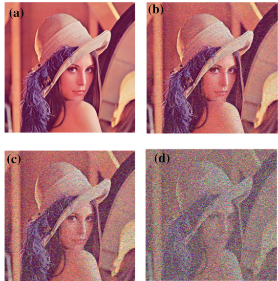
Fig. 18 Decrypted images with salt-and-pepper noise of various density n : a n = 0 , b n = 0.05 , c n = 0.1 , and d n = 0.2
