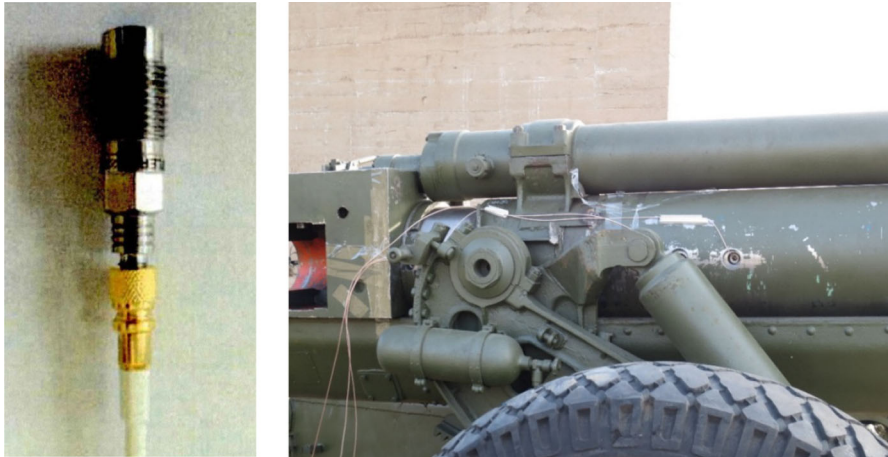
Fig. 10 Pressure sensor (left) and its locations on the test section (right)
