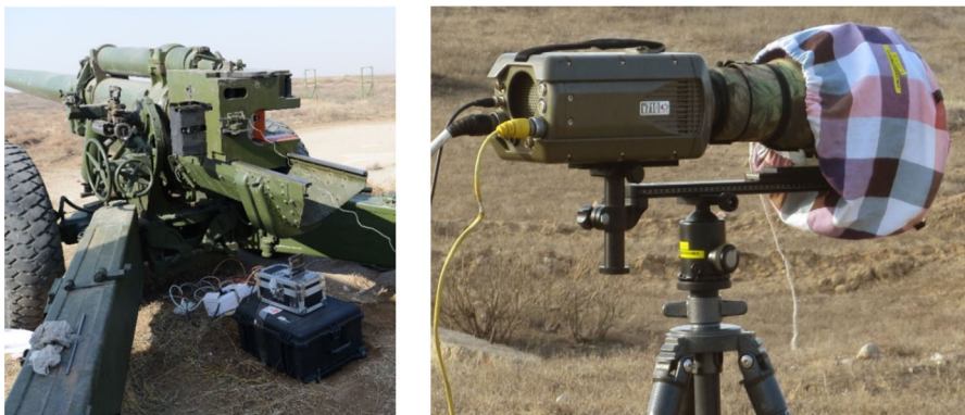
Fig. 11 High-speed photography system for artillery recoil movement
