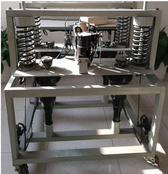
Fig. 11 The active suspension testbed
